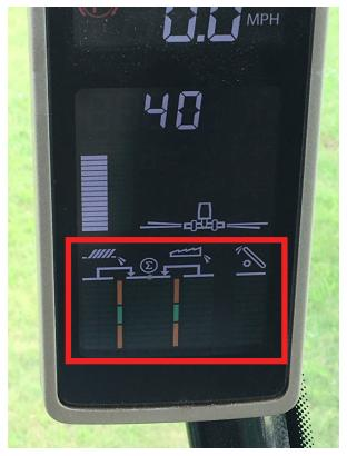
It includes Shoe and Separator Loss Monitors and Tailings Volume Monitor.
