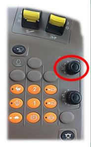
Height Sensing is enabled by selecting the Height Sensing option under Header Setup. Once the symbol is displayed on the cornerpost, this confirms it is active.
