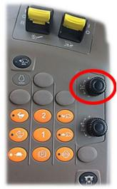
Header Resume must first be enabled by selecting the Header Height Resume box under Header Setup. When the symbol is displayed on cornerpost, this confirms it is active. Press the #3 button on the hydro handle- you will notice the number on the AHC panel of the Cornerpost.
